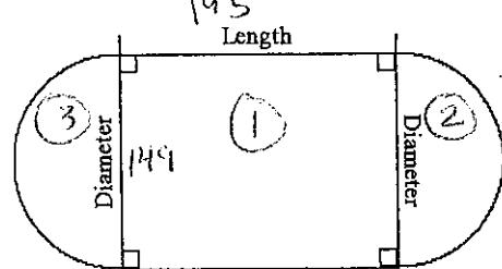
$$\begin{aligned} \textcircled{1} & 195 \times 149 = 29055 \\ \textcircled{2} & \frac{3.14 \times (74.5)^2}{2} = 8713.8925 \\ \textcircled{3} & 8713.8925 \end{aligned}$$
